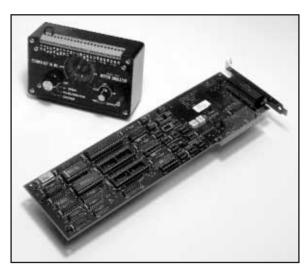
1-, 2-, or 3-Axis, High-Speed ISA-Bus Stepper Motor Controller
